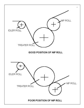
The nip roll must be supported by the base roll. (See good position of nip roll). With no support in locations below the diameter line - the nip roll will hang away from the base roll in the middle of the line and not achieve the intimate contact required to eliminate air. (See poor position of nip roll).
